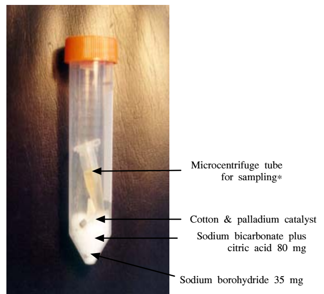
Figure 1. A photograph of the anaerobic pack devised for the transfer of T. vaginalis in this study. *Cap of microcentrifuge tube is pierced by needle for ventilation.
