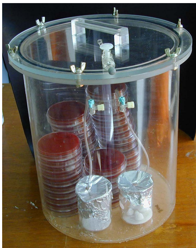
Figure 1. A photograph of the anaerobic jar devised for many plates culture of G. vaginalis in this study.
